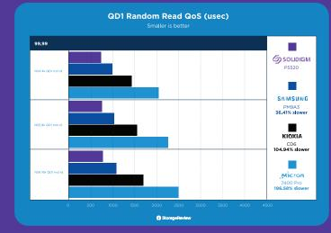
That gap increased, though, moving to the 99.99 percentile, where we started to see competing drives dramatically ramp up response times. Here the Solidigm D7-P5520 measured 769 microseconds, with the Samsung PM9A3 measuring 1,049, the Kioxia CD6 with 1,576, and the Micron 7400 Pro with 2,281.
