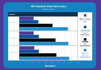
Moving to the six-9s or 99.9999 latency measurement, the D7-P5520 continued its impressive lead over the group, measuring 1,123 microseconds. The Samsung PM9A3 remained in second place, measuring 1,494, the Kioxia CD6 jumped to 2,748, and the Micron 7400 Pro measured a staggering 3,796.
