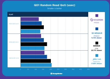
With more devices on the field, the Solidigm D7-P5520 held the lead for completion latency and 99.99 percentile and 99.9999 percentile latencies. Starting with completion latency (clat), the average of the D7-P5520 times across namespace 4-6 measured 141 microseconds, with the next closest being the Samsung PM9A3 with 157, followed by the Micron 7400 Pro with 166, and lastly, the Kioxia CD6 with 177.
